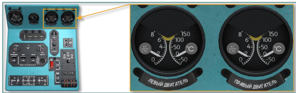
Рис. 9.54. Oil pressure/temperature gauges, center console
