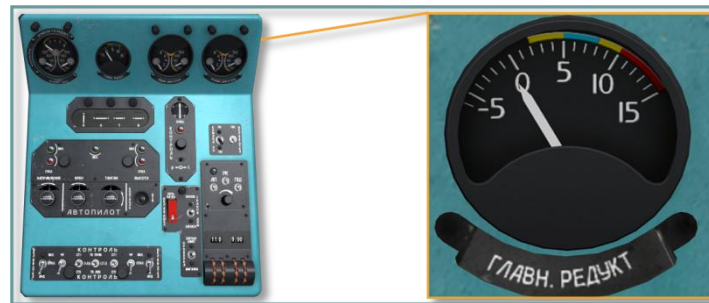
Рис. 9.58. Main transmission oil temp gauge, center console
