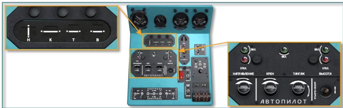
Рис. 9.88. Autopilot system control panels, center console
