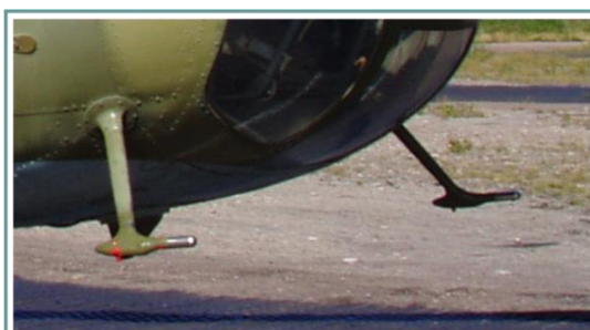
Рис. 9.69. Left and right pitot tubes
