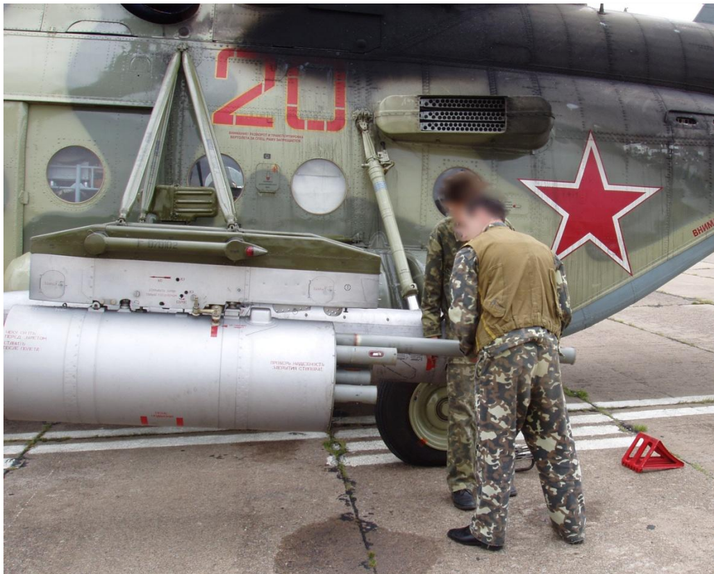
Рис.9.131. Loading of a B8V20-A rocket launcher on an Mi-8MTV5 helicopter.
