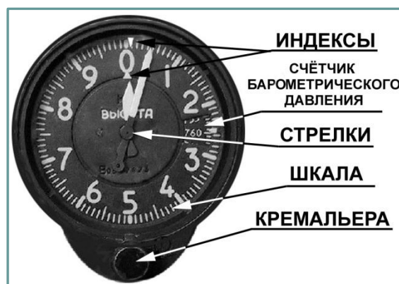
Рис. 9.75. Pressure altimeter function elements
