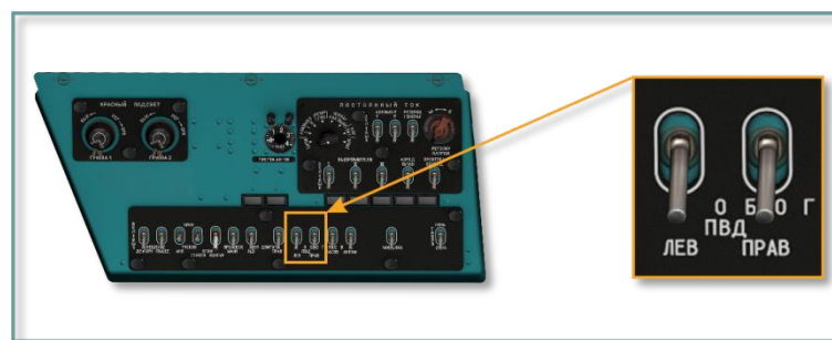
Рис. 9.70. Pitot tube heat switches, right side panel
