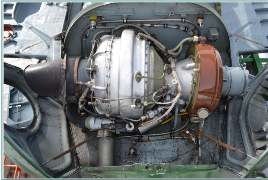
Рис. 9.26. AI-9V APU mounted on the helicopter
