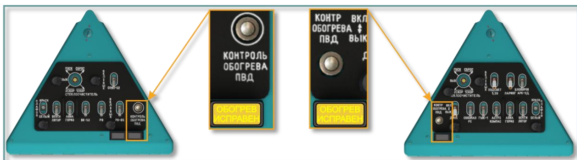
Рис. 9.72. Pitot heat test buttons and HEATER OK annunciators
