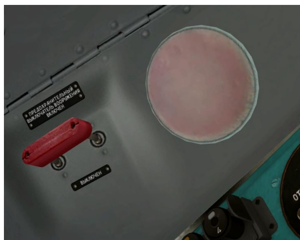
Рис. 9.123. The Master Arm switch and its associated red caution lamp.
