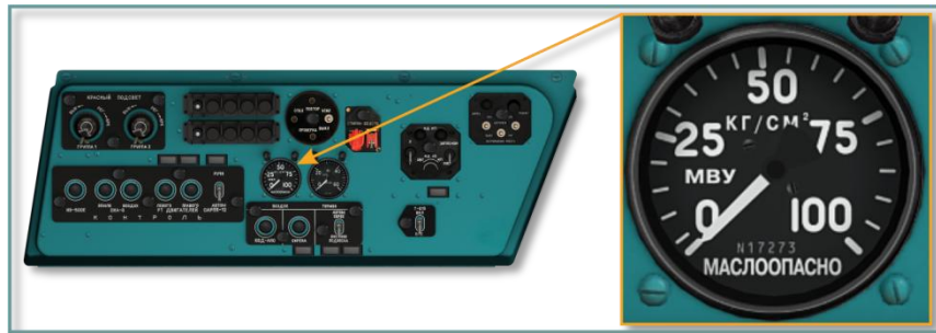
Рис. 9.66. Pneumatic system pressure gauge, left side panel
