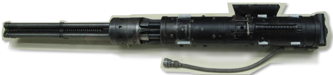
Рис. 9.140. YakB-12,7 12.7 mm 4-barrel Gatling gun
