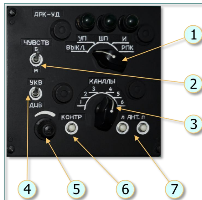
Рис. 9.101. ARK-UD control panel:
