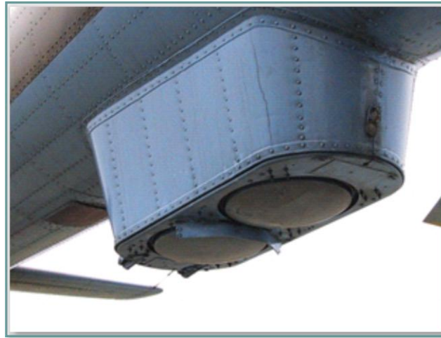
Рис. 9.102. DISS-15 high frequency unit
