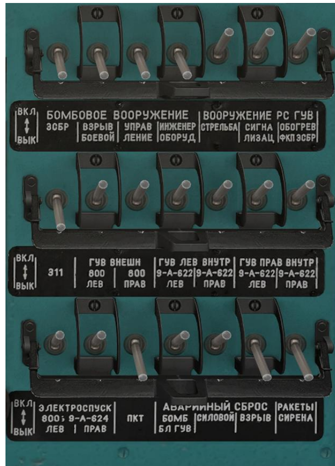
Рис. 9.122. Weapons Systems circuit-breakers.
