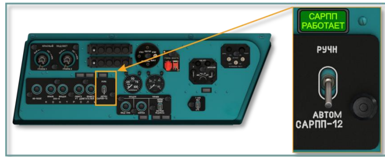
Рис. 9.68. SARPP-12D1M FDR power switch and indicator light, left side panel
