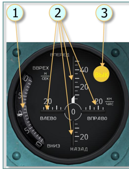
Рис. 9.104. Stationary flight indicator:
