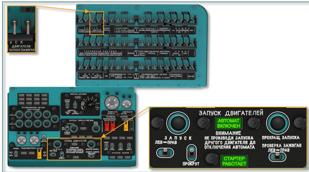
Рис. 9.29. Engine start control panel
