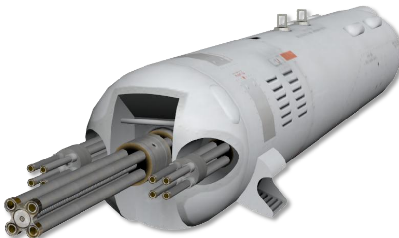
Рис. 9.137. GUV-1 equipped with automatic grenade launcher
