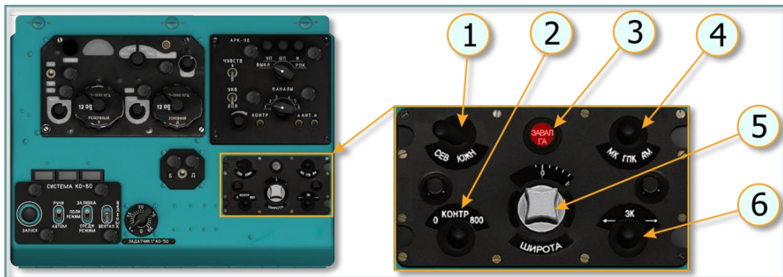
Рис. 9.81. PU-26 control panel, right overhead console:
