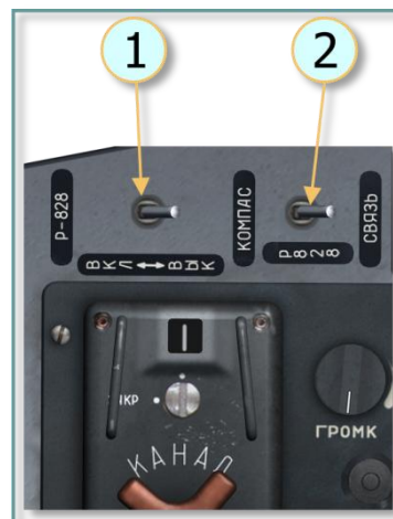
Рис. 9.96. R-828 power and mode switches:
