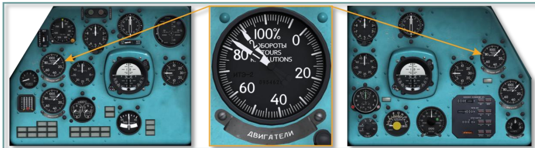
Рис. 9.52. Pilot's and copilot's dual engine tachometers
