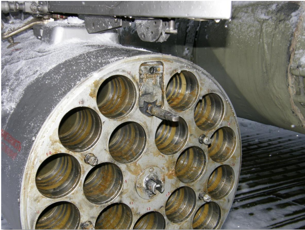
Рис.9.132.B8V20-A launcher tubes as seen from the rear.
