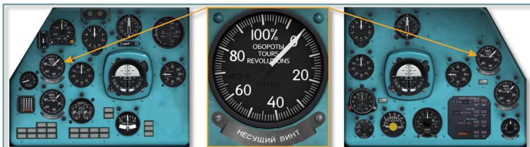
Рис. 9.53. Pilot's and copilot's main rotor tachometers
