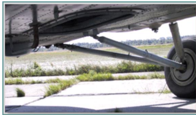
Рис. 9.94. NIPV-type antenna of the R-828 radio set
