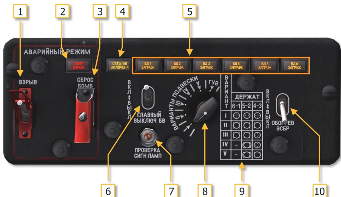
Рис. 9.126. Copilot's payload configuration panel
