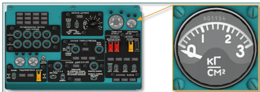
Рис. 9.61. APU air pressure gauge, center overhead console
