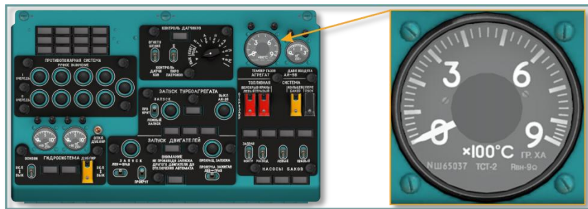
Рис. 9.60. APU EGT gauge, center overhead console
