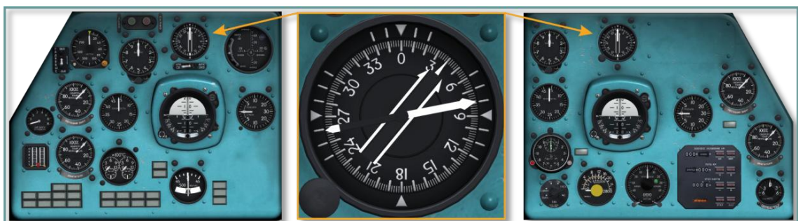
Рис. 9.82. UGR-4UK directional gyro
