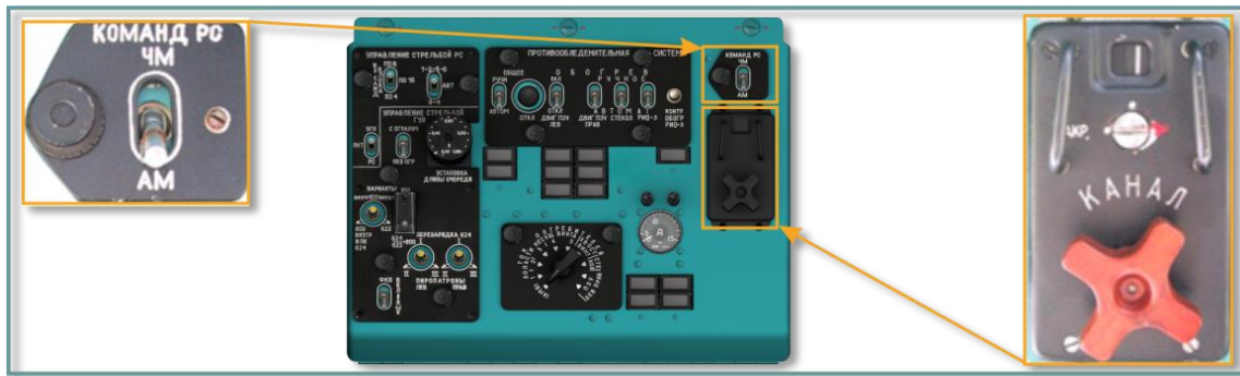
Рис. 9.90. Left overhead console: R-863 "КОМАНД. РС АМ-ЧМ" (AM-FM) switch (FM up position, AM down position); R-863 "КАНАЛ" (CHANNEL) selector panel with 20 available channels.
