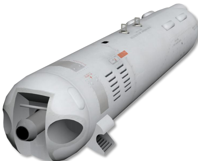
Рис. 9.137. GUV-1 equipped with automatic grenade launcher
