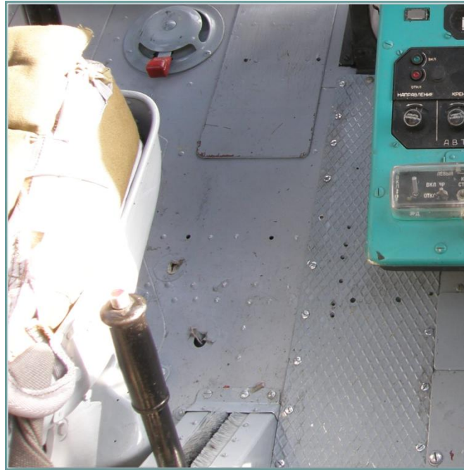
Рис. 9.31. Rotor brake control lever
