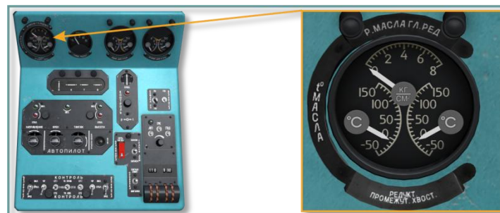
Рис. 9.55. Three pointer drive system oil pressure/temperature gauge, center console
