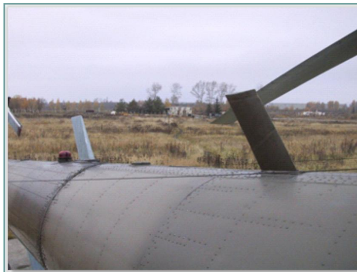
Рис. 9.100. AShS-UD blade antenna
