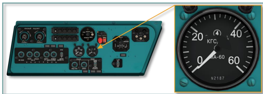
Рис. 9.67. Brake pressure gauge, left side panel
