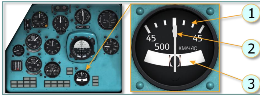
Рис. 9.79. Turn and slip indicator:
