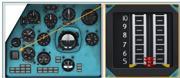
Рис. 9.57. Engine pressure ratio (EPR) indicator
